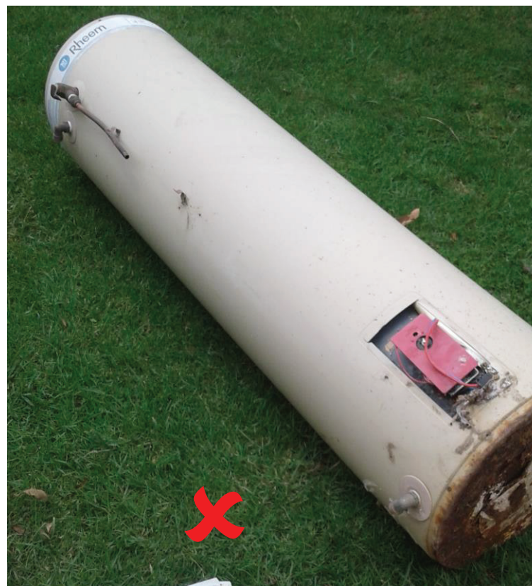
8 No hole in tank, element is intact
